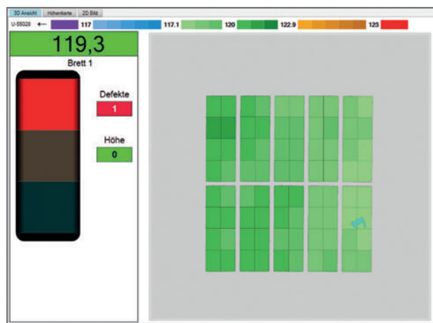
Results display with detection of surface cracks on the products.
