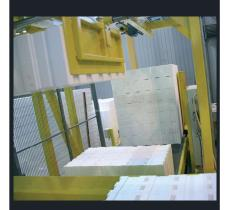
Automatic insulation feeder for concrete/insulation block production
