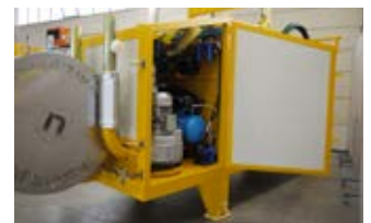
Vacuum assembly with sound insulated inspection panel
