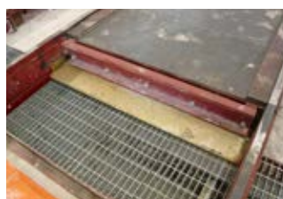
Safety grate for debris conveyor chain
