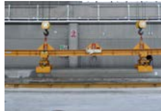
Double lifting hook for long lifting beams
