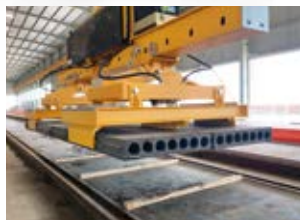
Hydraulic lifting clamps for wall panels
