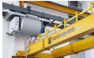
Fly bucket with the concrete distributor
