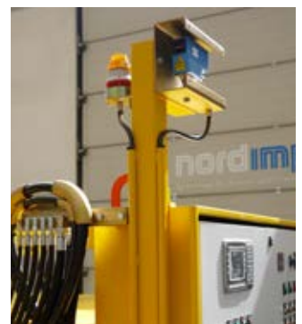
Laser device for automatic movement control
