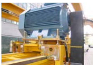
Electric motor and toothed drive belt to rotate
