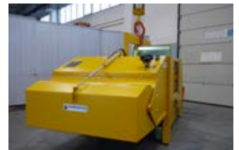
Container for collecting debris and water with hydraulically powered emptying
