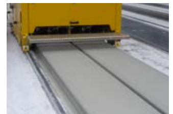
Production of 2x600 mm hollow core slabs
