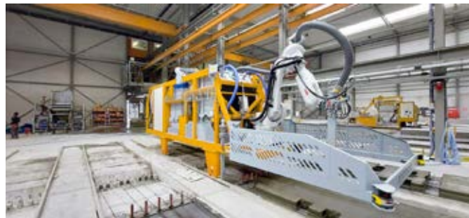
Automatic concrete aspirator
