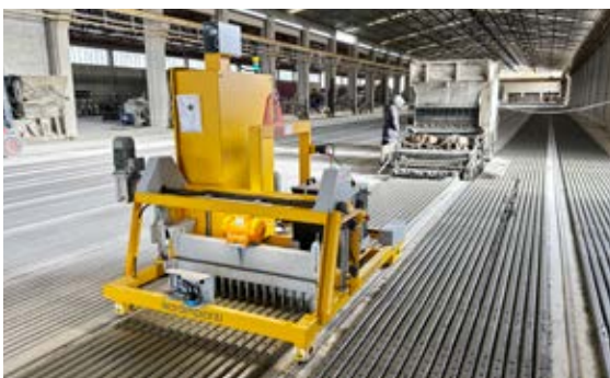
The machine follow the casting machine without the need of an operator
