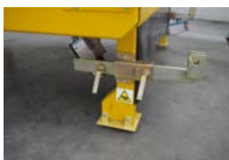
Connection between T-beam marking machine and saw
