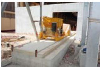
Trolley during the bucket transport from the batching plant to the production area
