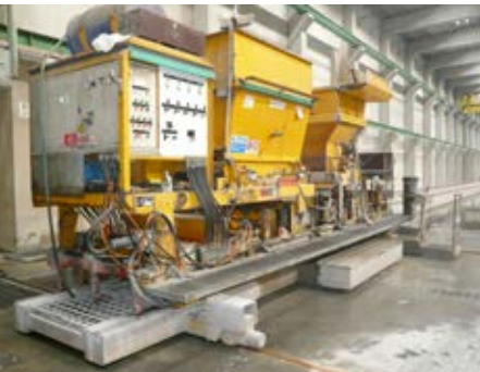
Casting machine being transferred from one bed to another without the need of an overhead crane
