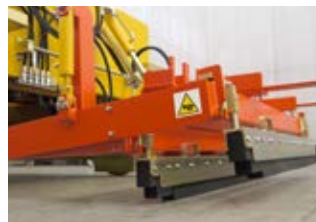
Replaceable squeegee for water collecting
