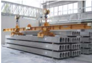
Mechanical lifting beam for hollow core slabs
