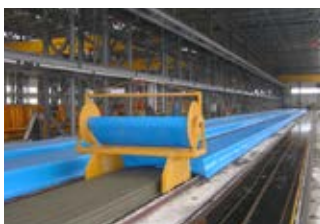
Coiler holding trolley Manual type
