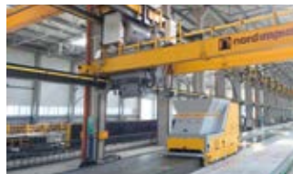
Fly bucket filling the concrete distributor
