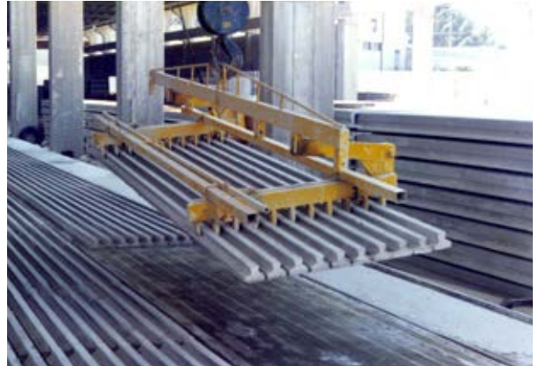
Mechanical lifting beam for inverted T-beams
