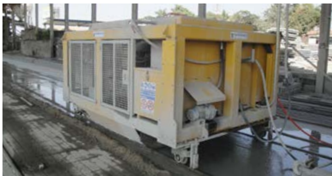
Milling machine for concrete beds
