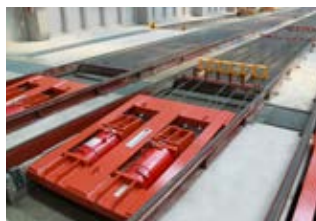
The detensioning cylinders installed in the reaction beams
