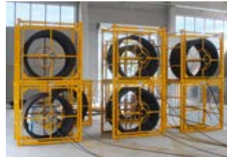
Stackable decoilers for strands or 2-3 wires
