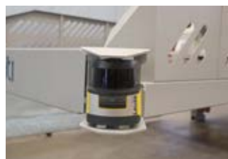
Scanning laser safety sensor
