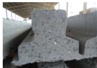
Element with uneven lower surface produced on a worn bed
