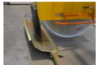
Casting for cutting water collecting
