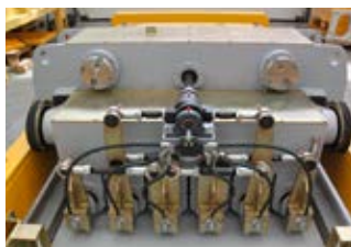
Gear box in a constant oil bath
