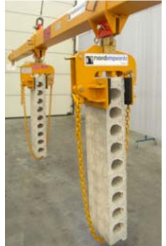
Ability to change the clamps to lift hollow core wall panels
