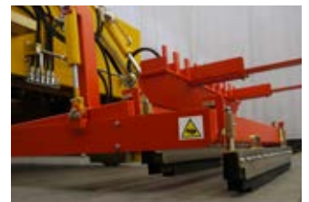
Replaceable squeegee to spread the detaching oil
