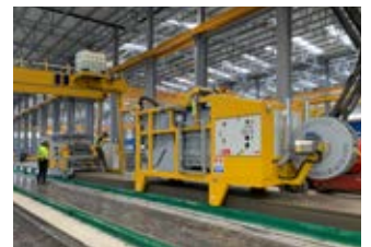
Concrete aspirator working behind the casting machine
