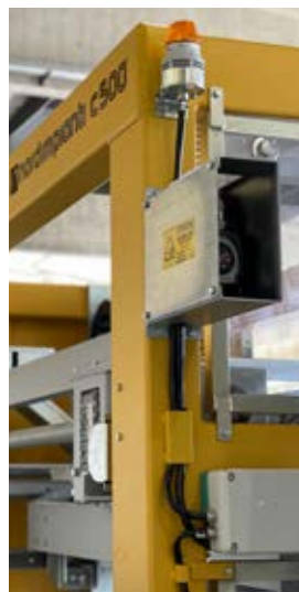
Laser device for automatic movement control
