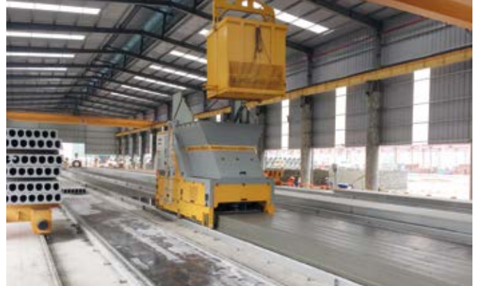
Concrete discharge into the hopper of the casting machine
