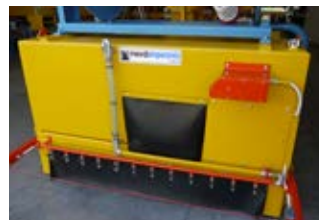
Water tank to apply water to the production bed using drippers, during the cleaning phase
