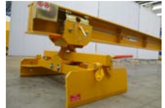
Pair of clamps with opening closing mechanism complete with safety chains
