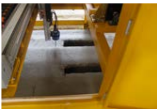
Inkjet head for during the element marking phase
