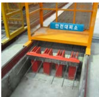
Reaction beam (tensioning side)
