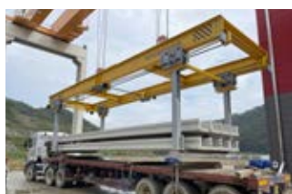
Able to handle any kind of precast element up to 2.4m wide
