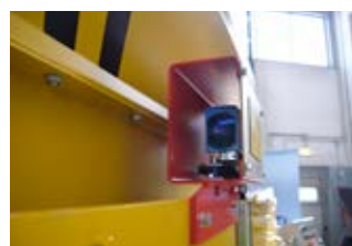
Laser for accurate positioning
