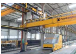
Fly bucket filling the concrete distributor
