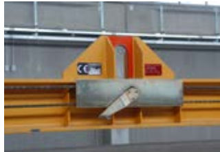
Clamp distance adjustable over the length of the beam
