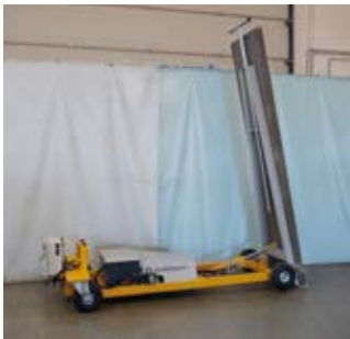
Trolley in the mounting position of the wall panel
