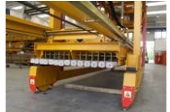
Interchangeable lifting clamps depending on the element to be lifted
