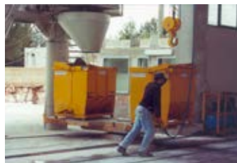
Bucket being loaded under the mixer
