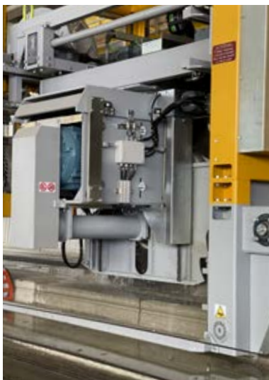
Double protection shield (one mobile and one fixed) for protection when the cutting blade is in operation
