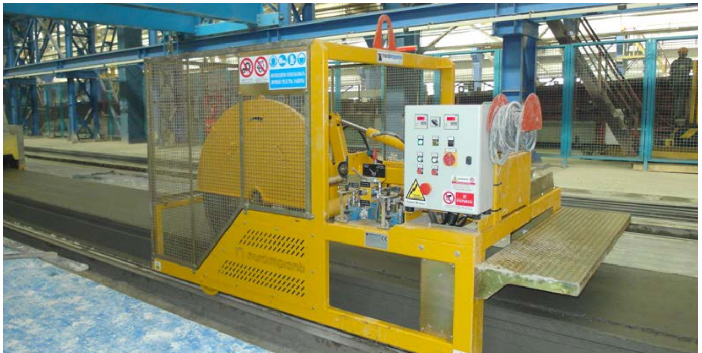
Hollow core slabs longitudinally cut by fresh concrete saw
