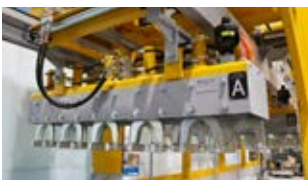
Lifting clamps actioned hydraulically
