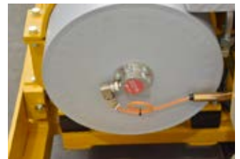
Load cell installed on the stressing cylinders
