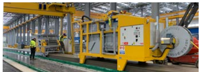
Concrete aspirator working behind the casting machine
