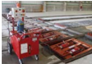
Detensioning pump unit connected to detensioning cylinders
