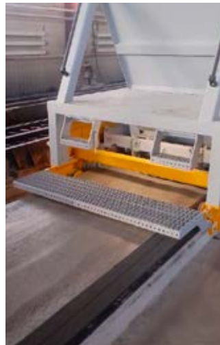
Production of 1200mm hollow core slabs
