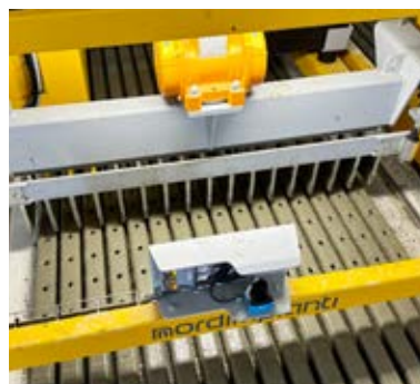
Safety laser scanner for automati movement
