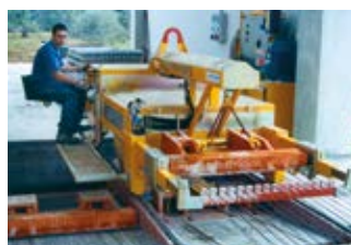
Equipment to lift the movable anchor (Optional)
