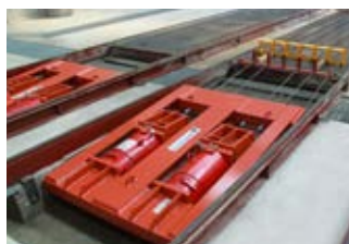
Reaction beam (detensioning side)
