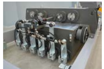
Gear box in a constant oil bath
