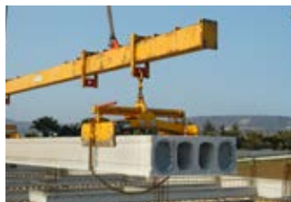
Clamps with opening and closing mechanism complete with safety chains
