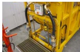
Side vacuum pipes for rail cleaning (Optional)
