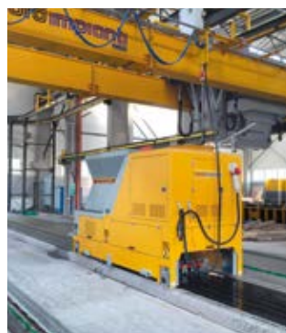
Electrical supply from the concrete distributor
