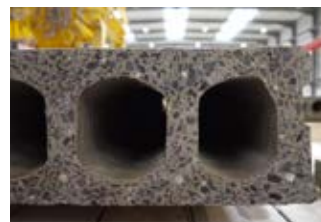
Excellent concrete compaction and steel wire bonding
