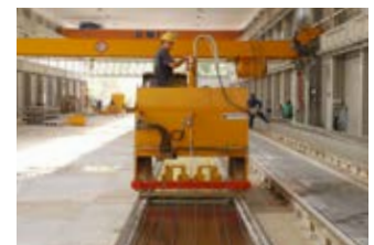
Bar to lay the steel wires
