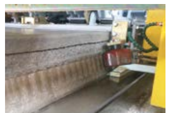
Para-seismic side indenting device (Optional)
